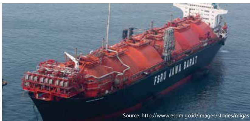
Fig.2. FSRU type of discharge terminal
